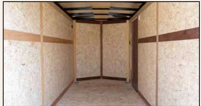
Deluxe interior shown with 3/8" PlexCore Sidewall Liner & 5,000 lb. Floor D-Rings.
