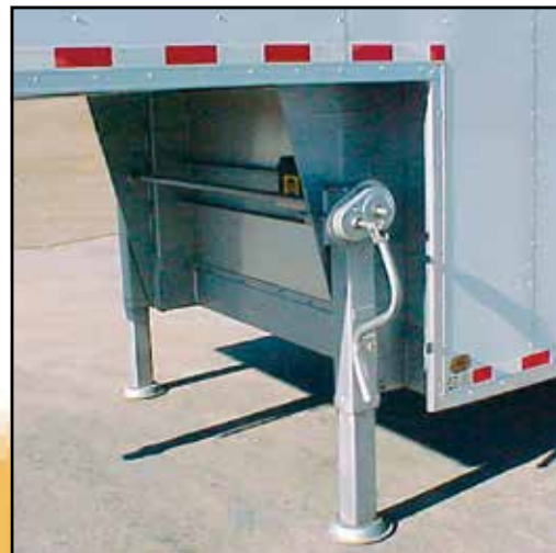
Tandem, 2-Speed Landing Gear: The dual gear ratio crank makes raising/lowering your trailer much easier especially with heavier payloads.
