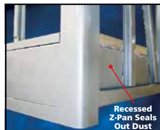
Flush Floor Installation Will Not Snag Cargo
