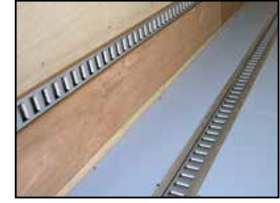
Cargo Control Systems (E-Track)
